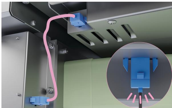
3. Ensure all cables click into place and are routed away from cooktop exhausts. Secure to cabinetry using the supplied harness retainers.
