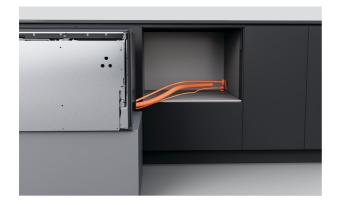
1. Place hoses and cords through the service holes and into the adjacent cavity.
