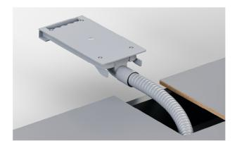
**3.** Pull the end of the venting hose through the cut-out and firmly attach it to the vent duct.
