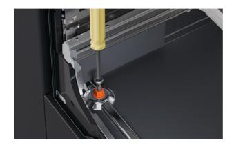
**5.** Insert the supplied 38mm screws and washers through the front two holes on the bottom of the chassis.
