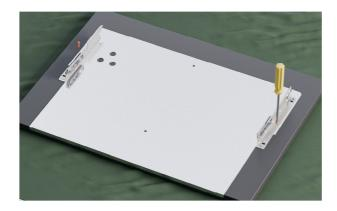
**5.** Fix one screw in each side through the bracket fixing points.
