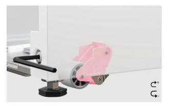
**4.** Using the supplied 6mm hex key, rotate counter-clockwise to raise both sets of wheels via the adjustment screws.
