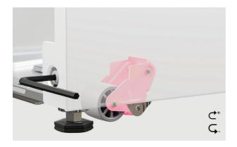
2. Partially roll stacked products into alcove and check alignment. To do this, use the supplied 6mm hex key, rotate clockwise to lower both sets of wheels via the adjustment screws.
