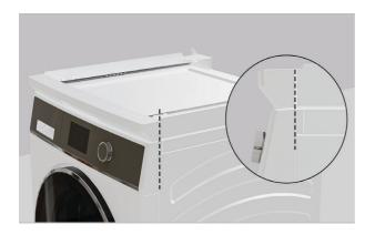
**1.** Align the front corner of the stacking kit to the washer.
