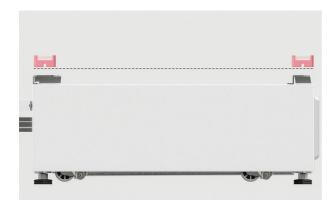
2. Place the plinth in its final install location. Adjust the feet using the supplied spanner until the washer is level front to back and corner to corner.
