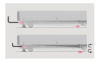
1. Open the cabinet door and lower the rear wheel using the supplied Allen key.
