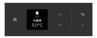
1. Press ✓ or ∧ to select the lower compartment, then press ✓ to confirm.
