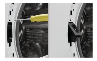
**4.** Unscrew latch, and slide to remove.
