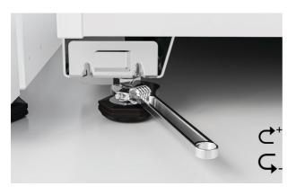
8. With cabinet in the final position, unscrew front levelling feet using the provided spanner. Re-check clearances and alignment before tightening the locking nuts up to the base of the cabinet to lock the feet into position.
