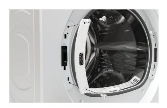
**3.** On dryer, unscrew and remove latch cover to access latch.
