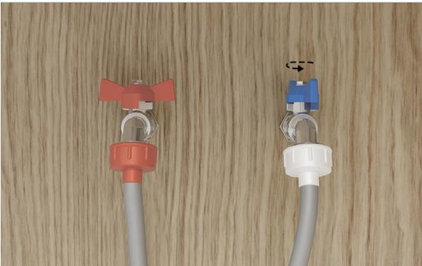
**8.** Connect hoses to taps before turning on. Check for leaks at all connection points. If possible, recheck for leaks 24 hours after installation.
