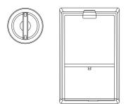
The salt reservoir is located on the inside of the drawer next to the detergent dispenser. It holds up to approximately 400g of salt (actual capacity will vary depending on brand and grain size of salt used).
