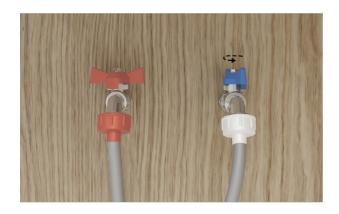
**4.** Turn off cold water tap for washer, and undo washer cold hose at tap end.
