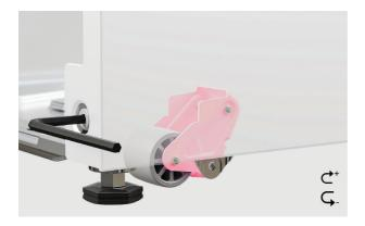
1. Partially roll stacked products into alcove and check alignment. To do this, use the supplied 6mm hex key, rotate clockwise to lower both sets of wheels via the adjustment screws.
