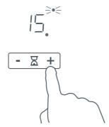
3 Set the time while the small red light in the bottom corner of the minute display is on. The timer is now set for the right rear cooking zone.
