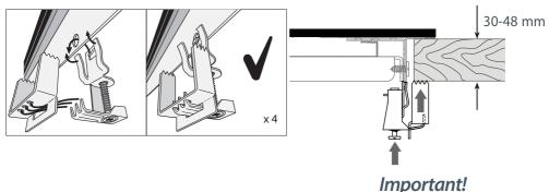
Do not overtighten the screws!
