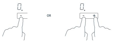
**1a Turn the cooking zone off** by scrolling down to  $\square$  or touching – and + together. Make sure the display shows  $\square$ .
