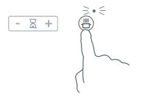
1 With the cooktop turned on, touch the PowerBoost control . The flashing red light indicates that PowerBoost is ready to be set.
