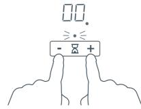
2 Touch the – and + controls of the timer together. The minute minder indicator will start flashing and 2 2 will show in the minute display.
