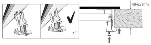
Important! Do not overtighten the screws!
