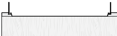
CUSTOM TOE KICK PANEL ALIGNMENT FOR 56MM TO 120M DEPTH
