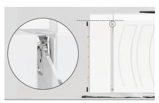
**6.** Ensure plinth is aligned on both sides as shown before tightening the front bolts with the supplied spanner.
