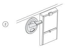
Attach the salt funnel to the DishDrawer<sup>TM</sup> Dishwasher and carefully pour salt into the reservoir.
