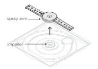
Lift the spray arm off the impeller, pulling up from the centre. Shake to dislodge any loose particles, rinse under running water and wipe with a damp cloth. Ensure the magnet is clean and clear and that water can flow through all holes.
