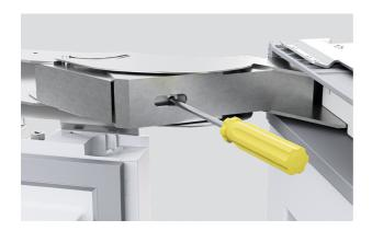
1. Release the hinge spring by turning the T20 screw in the hinge to the 'O' position. Close the door and lay the appliance on its back on the pallet.
