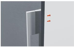
**3.** Fit the handle to the panel using four M5x25 hex screws.
