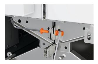
2. Secure the lower brackets together using the supplied M6 screw and Nut. Secure using a 4mm Allen key and 10mm spanner.
