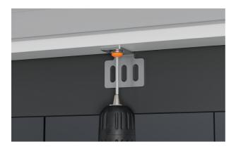
1. With the door open, loosen the lower bracket screw. Adjust bracket to rest against the door panel. Re-tighten the bracket screw.
