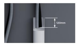
**5.** Ensure the hoses do not extend more than 120mm into the standpipe to prevent wastewater siphoning back into the tub.
