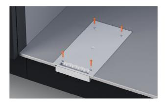
**4.** Secure the vent using the provided screws.
