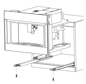
3 Position the appliance on the rails, making sure the pins are correctly inserted in the housings, then fix it with the screws supplied. If the height of the appliance requires adjusting, use the spacer disks provided.
