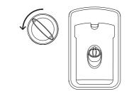
Turn the cap anticlockwise and remove.
