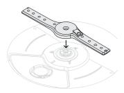
Place the spray arm to the impeller. Ensure the arm rotates freely when refitted.
