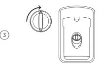
Refit the cap, turning clockwise until secure.
