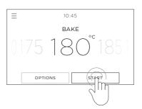
To adjust the preset temperature, swipe left or right or use the dial. Touch **START** to heat the oven and begin cooking.
