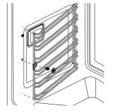
Fit the side rack front tab over the fixing screw.
