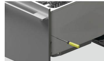
Insert a crosshead driver into the hole above each side pin and rotate to adjust the panel alignment. There is a maximum travel distance of  $\pm 1/16"$  (2mm).
