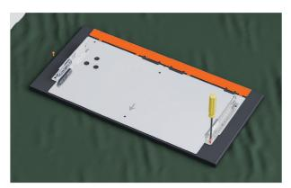
**6.** Remove the door panel and fix the remaining four screws. Bend the top of the bracket back and forth until it snaps off.
