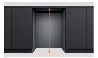
**2.** Measure the distance from the floor to the underside of the countertop or cavity frame.
