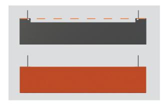
**4.** For a toe kick depth up to 40mm, align the top of the custom panel to the top edge of the toe kick mount.
