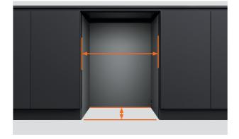
**2.** Ensure the cabinet meets the minimum cavity specifications required.
