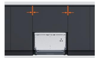
**2.** Subtract the required gap between the cabinet panels from each measurement.
