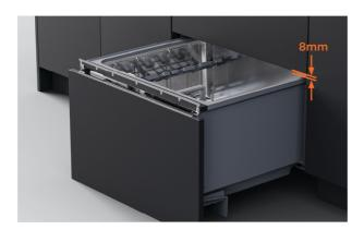
5. Slot panel onto dishwasher. Check that the gaps between the panel and adjacent cabinet doors are a minimum of 2mm. Check that the gap between the top and bottom drawer panels is a minimum of 8mm for ventilation.
