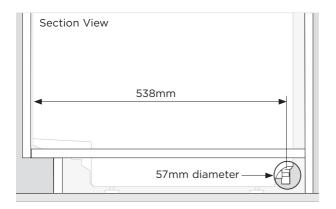
1. A minimum 57mm diameter service hole is required in the cabinet side.
