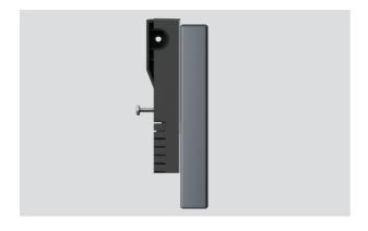
**6.** Drill pilot holes through fixing points in the toe kick mount.
